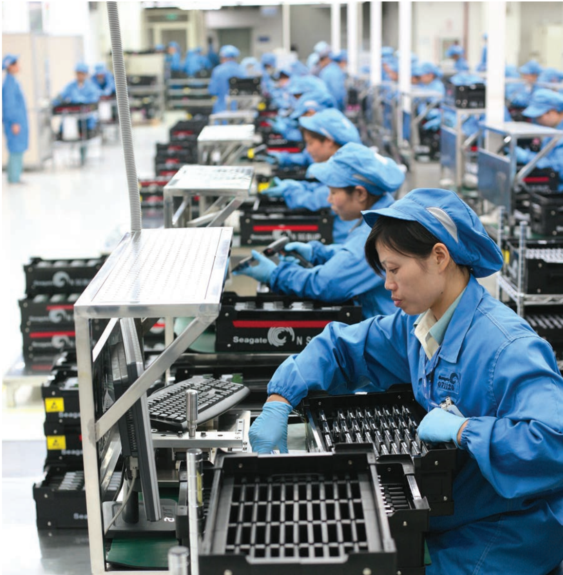
Workers perform final testing and QA before sending drives off to customers on its 2.5-inch notebook lines at Seagate Wuxi Factory." (Robert Scoble, November 6, 2008)
